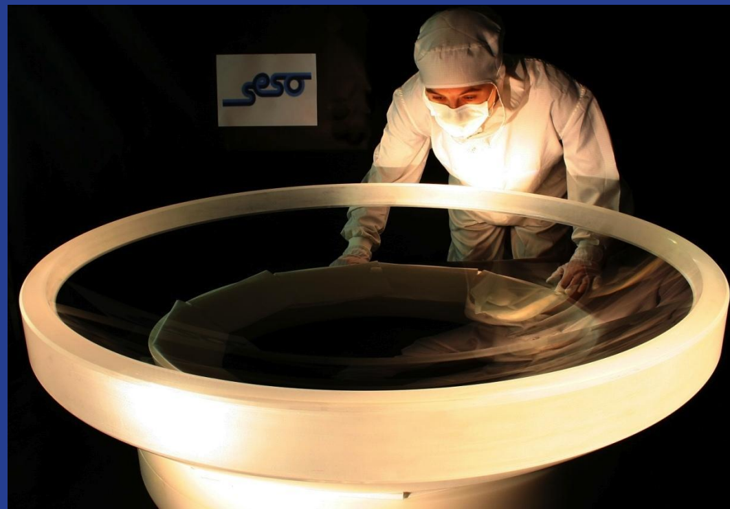
Steve Kent inspecting the C1 Blank (980mm diameter) at Corning New York Jan. 2008
