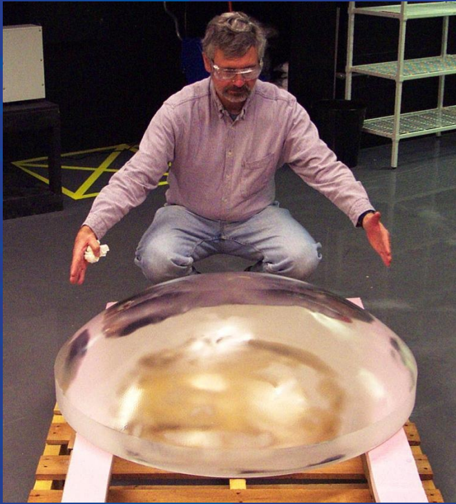
Steve Kent inspecting the C1 Blank (980mm diameter) at Corning New York Jan. 2008
