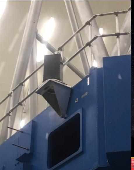
On-sky test to measure the deflection of the optical axis of the LPC due to the relative flexure with respect to the optical axis
