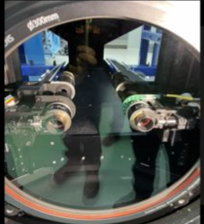
GHOST Cassegrain acquisition unit showing the mini-IFU arms.
