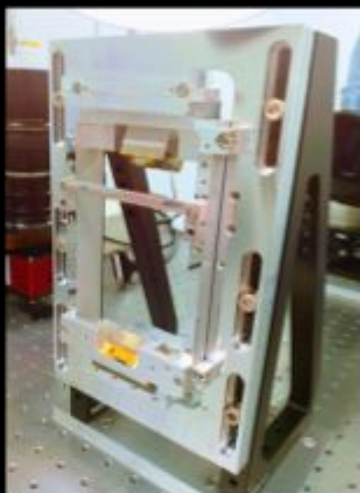
Assembled LR IFU. F2 & F3 fore-optics (left) and S1 slicer (right).
