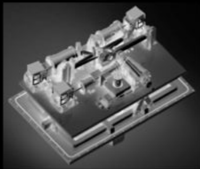
IGRINS-2 3D model. On the top the H & K arms, on the bottom the IO and SVC.
