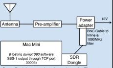
Cerro Pachón ground station schematic. The antenna and pre-amp are located on top of the ALO building at the LSST site, and are connected to the power adapter indoors by a coax cable
