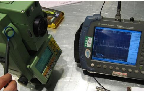
EMI leakage measurement: gap of the pillar, screen and lens
