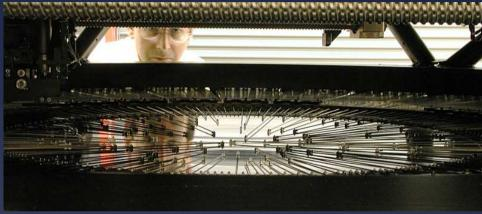
Hectospec – PI: Dan Fabricant 300 1.5 arcsec fibers over a 1 degree field – these feed one of two spectrographs with resolution of 1000 (3700-9200A), and 30,000 (150A per order)
