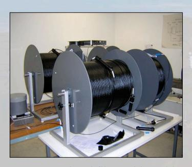
2x300 m K band fiber cables with 6 sections (0.1 dB loss per connection)
