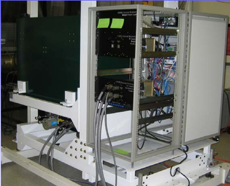
OSIRIS: OH-Suppressing Infra-Red Imaging Spectrograph UCLA Infrared Imaging Detector Laboratory James Larkin, PI
