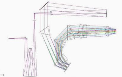
Optical layout of FIRE, showing 1:1 pre-slit Offner relay, reflecting collimator, cross-dispersing prism array, reflective diffraction grating, and four-element camera. (R. Bernstein)
