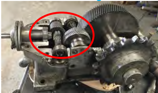
Dome drive gear box before & after refurbishment
