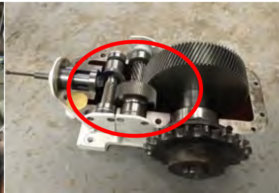
Dome drive gear box before & after refurbishment
