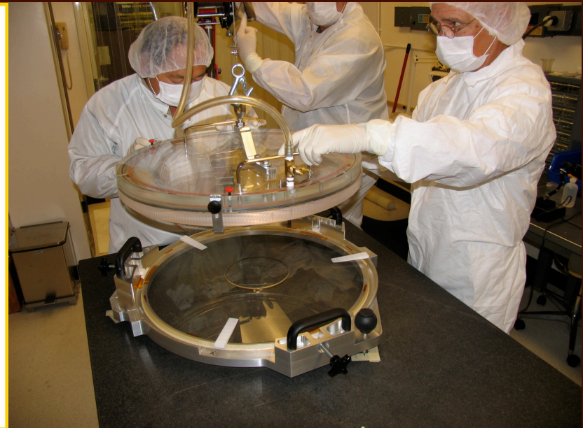
ODI ADC under construction
