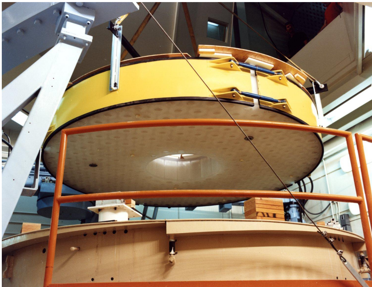
Caption: The underside of the mirror, supported by the now finished handling band, painted yellow
