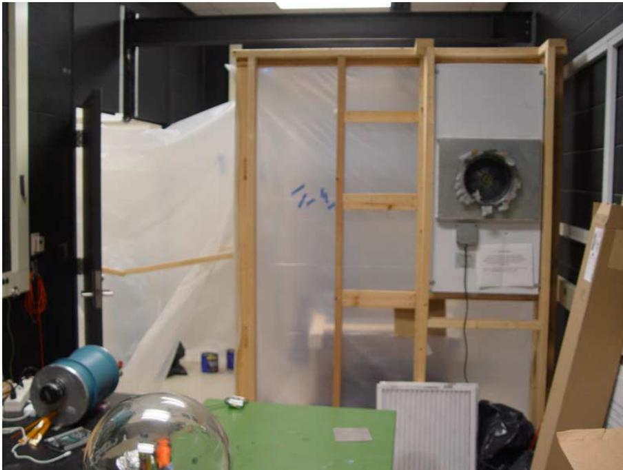
Figure 1: Clean room. The ante room is at the left. The filter-fan module is at the right. The rail (black) for the hoist is above.
