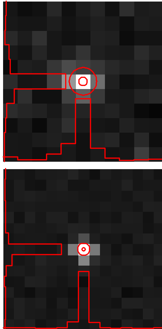
Figure 1 Images 1 in the f/21 channel (top) and the f/12 channel (bottom) of an 8- \mu m pinhole illuminated with a 632-nm laser. The geometrical image of the pinhole is the smaller circle. The first dark diffraction ring for 632 nm is the larger circle, which is twice as large for the J band.
