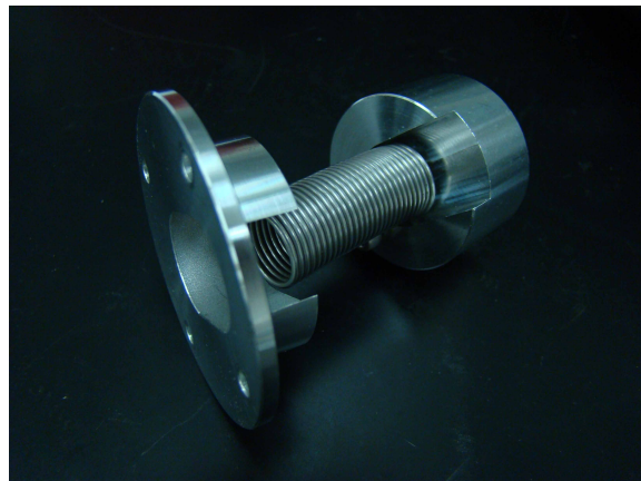
Figure 8: Arborless antibacklash mechanism for the wheels. The base is on the right.
