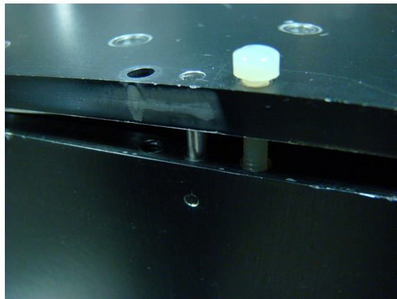
Figure 7: Lifting the top plate of the COB. The nylon screw lifts the top plate and frees it from the pin.
