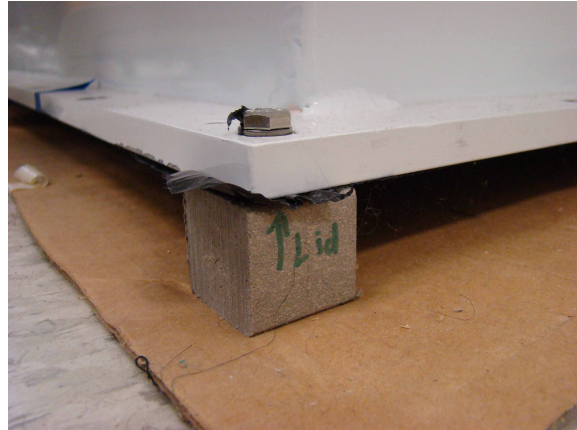
Figure 4: Vacuum lid showing a wood composite foot (gray). Shreds of the protective cover, a black garbage bag, show between the lid and foot.
