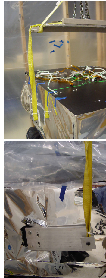
Figure 6: Top: Spreader bar and offset plate of the turning jig. The cable tie keeps the strap on the spreader bar. Bottom: offset plate attached to the A-to-C transition. The strap guide and the cable tie prevent the strap from slipping off the black shoulder bolt.
