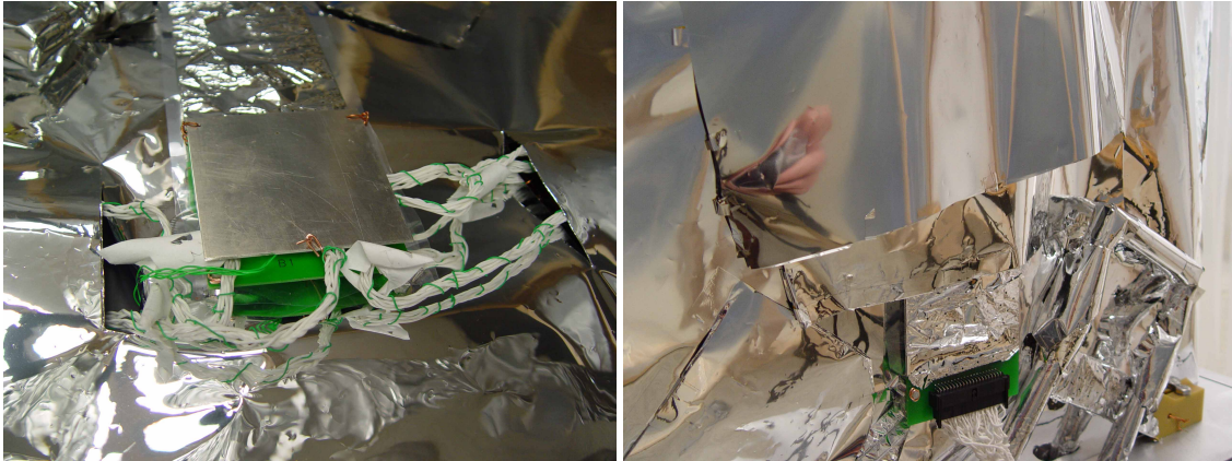
Figure 10: Left: Cover (the aluminum plate) for the motor board. Right: Double layers of aluminized Kapton covers the cold end of the motor board. The warm end, which has the wide cable, is uncovered.
