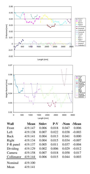
Figure 7: Top and bottom edges (top panel) and height (middle panel) of the walls. Each wall is positioned where it connects to the previous one. Table at bottom contains the heights of the walls.
