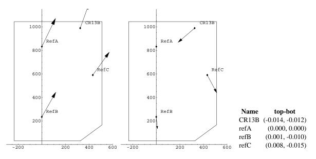
Figure 6: Shift (left), magnified by 3000, of the pins in the top plate with respect to those in the bottom. Shift (right), magnified by 10,000, after offsetting by the shift of refA (0.038, 0.079). Residuals (in Table) are calculated after offsetting.
