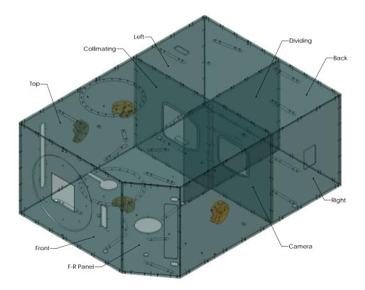
Figure 1: The cryo-optical box. Each optic attaches to both the top and bottom plates. The walls keep the top and bottom rigid.
