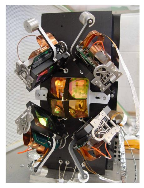
Figure 13: 4-eye detector assembly. Each detector butts against a frame and outer frame, for two of which the field-flattening lenses are visible. Each outer frame mates to two Henein axles, a complicated, shiny object. Each pair of Henein axles mate to a leg, and legs mount to the spine, the black object in the back.
