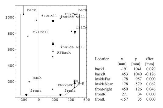
Figure 5: Deviation, magnified by 2000, of the bottom edge of the walls from a plane. An down arrow indicates the wall is low (shifted away from the top). The right edge of the back wall is low (shifted away from the top) by 0.13 mm. The asterisks show the location of the optics, the mask, f/21 collimator, f/12 collimator, the filter-fold mirror assembly (FFFront and FFBack), f/21 camera mirror, f/12 camera mirror, and detector assembly (dA).
