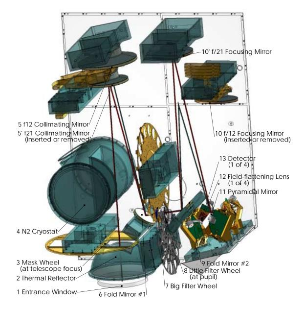
Figure 2: Optical schematic. These parts require alignment: the mask assembly (3), the two collimators (5 and 5'), the filter-fold assembly (6–9), the two camera mirrors (10 and 10'), and the detector assembly (11-13).
