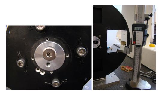
Figure 8: Left: Use of the cen-o-matic to center the mask wheel on the rotation stage. Right: Use of a height gauge to find the reference position of the mask wheel.
