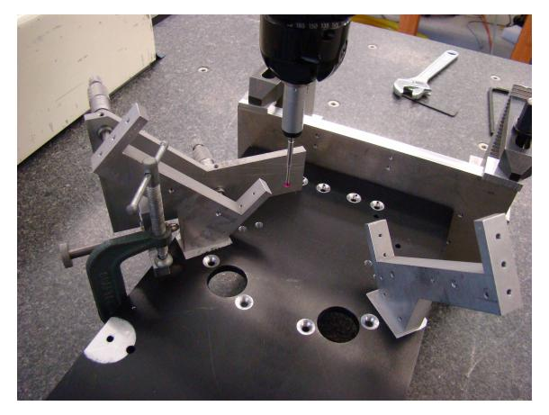
Figure 14: Alignment of 4-eye showing a nudger and two micrometers used to position the leg for detector A1. The spine is bolted on the faux COB, which is clamped to the bed of the coordinate-measuring machine.
