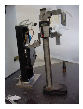
Figure 12: Use of a height gauge to set the rotation of the mirror arm for the high-res collimator
