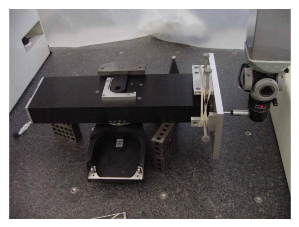
Figure 11: Alignment of the shims (one is visible on the left) on the high-res collimator mechanism with the pads (three shiny regions on the mirror arm) and pins (in which tooling balls are inserted) for the mirror. A nudger is attached to the shim on the right.
