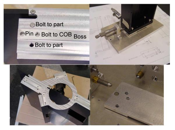
Figure 3: Bottom left panel: the bottom shim for the fold-filter assembly. (The shim is shiny.) Top left: detail showing the region of shim near the large filter wheel. Right panels: faux COB for positioning the assembly.
