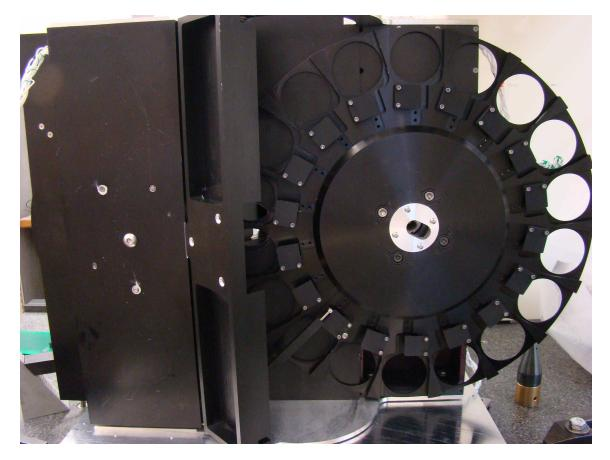
Figure 10: Filter-fold assembly with the top shim (shiny, curved part) bolted on the alignment jig. From left to right are the cradle for the little filter wheel, the post for fold mirror #1, and the big filter wheel.
