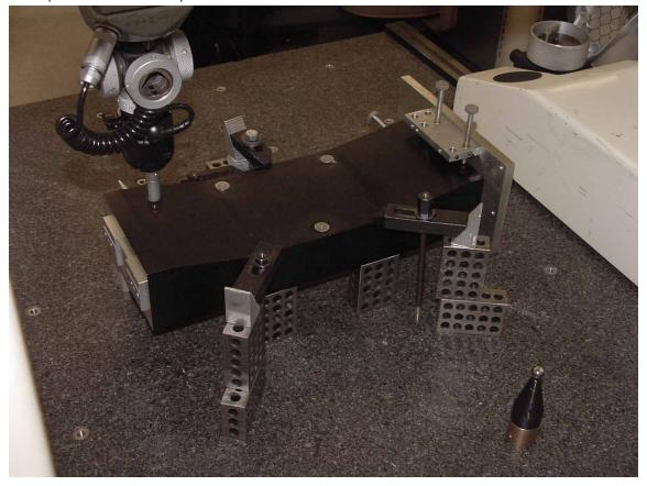
Figure 9: Alignment of the shims (one is visible on the left) on the wide-field collimator post with the pads (three shiny circles) and pins (too small to be seen) for the mirror. Three nudgers are attached to the faux COB to move the shim on the right.
