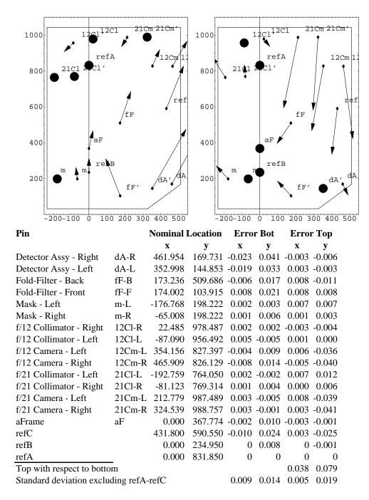
Figure 4: Errors (magnified by 10,000) of the pin holes in the bottom (left panel) and top (right panel) plates. Points with errors less than 0.005 mm are shown as dots. The points are shifted so that refA has zero error and rotated so that refB has minimal error.
