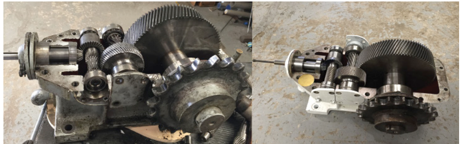
Figure 1: Reduction gearbox for Blanco dome azimuth drive before (left) and after (right) repair. (Image credit: Andrés Montané/NOAO/AURA/NSF.)
