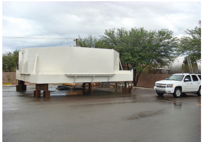
Figure 9: The delivered shipping/storage container for the LSST M1/M3 mirror.
