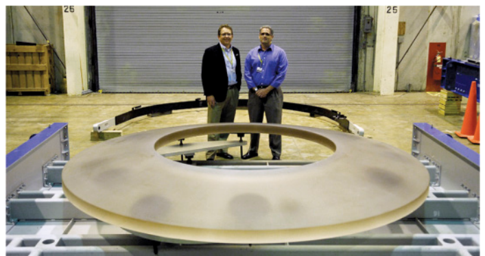
Figure 1: Victor Krabbendam (left) and Bill Gressler (right) stand behind the LSST M2 substrate, which is in its shipping/turnover fixture.
