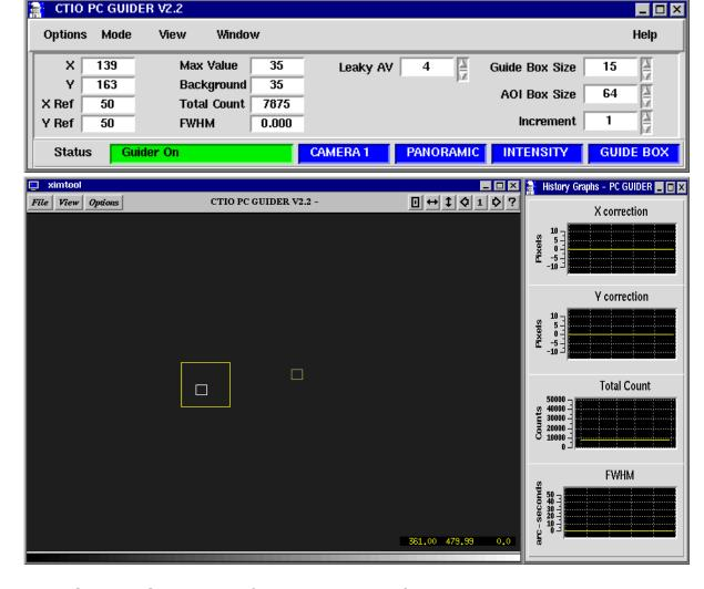
The PC guider GUI consist of one main window from which the most common operations (e.g. turning the guider on) are initiated, a history graphs window, and the display server window. Eventually some other auxiliary windows can be popped up as well.
