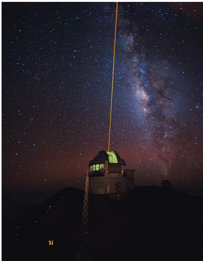
Gemini-North with its Laser Guide Star (LGS) system in operation. The exposure time for this picture was one minute and was taken during commissioning in July 2006.
