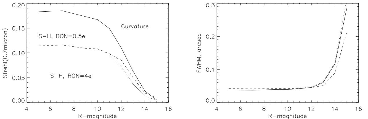
Figure 1: Strehl ratio (left) and FWHM (right) against guide star R-magnitude. Full line: curvature system, 1 ms loop. Dashed line: S-H system, 2 ms loop, 2x2 pixel/subap. WFS, RON=0.5e. Dotted: same, RON=4e.
