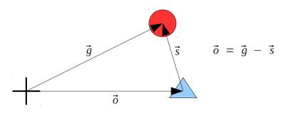
*Figure 8:* The cross mark the telescope coordinates in the sky-map. The circle is the selected star. The triangle is the field center.
