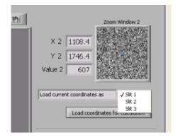
Do not forget to switch the number of the slit before you load the coordinates for calculation. Often times, for the alignment boxes, it is easier to find the centroid by eye instead of using the centroiding algorithm.
