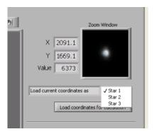
Repeat the same procedure for Star 2. Then send the coordinates to the calculator. Again, use the drop down menu to switch from Star 2 to Star 3, then find and load the coordinates for the third star and send then to the calculator.
