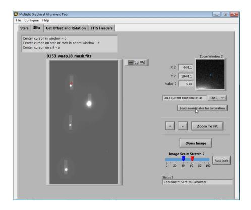
Now, use the "Open Image" button to open the image of the MOS mask. Again, the image is located in the current directory. Click "Zoom to Fit" and "Autoscale" after you open the image. If the scaling is not useful, you can use the red and blue sliders to adjust the scaling of the images.
