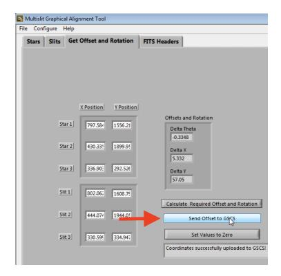
This sends the offset coordinates to the main GUI panel. On the main GSCS Panel, click "Calculate the required offset".
