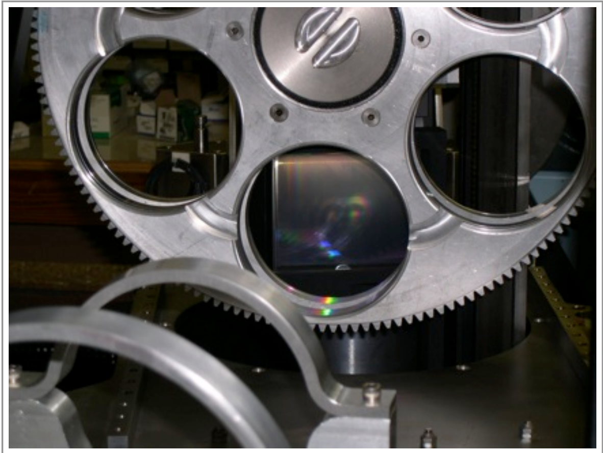
Figure 7: View from the collimator (removed) looking through the filter wheels into the grating.
