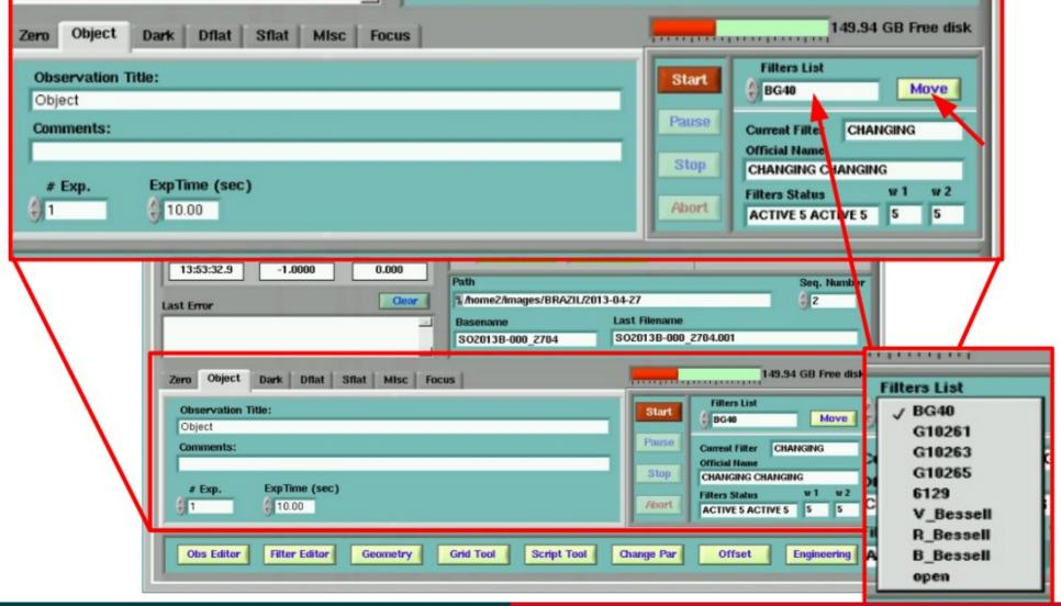
Select the appropriate tab depending on the exposure type. This information will go into the image header keyword **OBSTYPE.**
