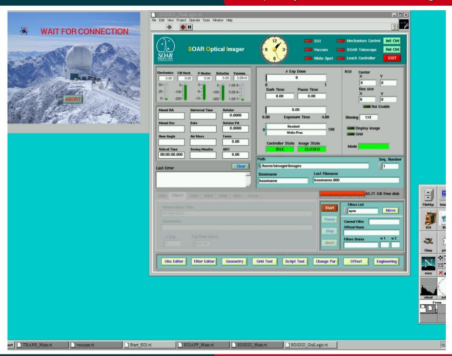
Labview applications need you to click on the upper left arrow to run them. Once the SOI GUI is up and running this is what it looks like. All your connection LEDs in the upper right should be green, and overall no error messages should show up
