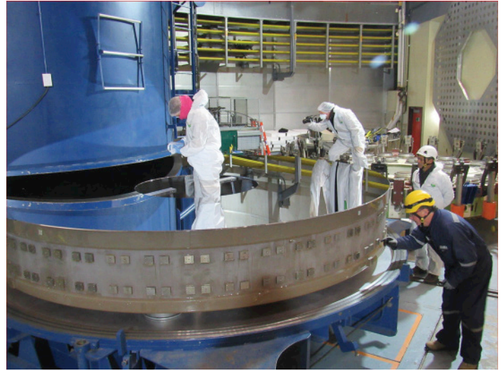
Figure 2. Inspecting the newly coated primary mirror as it is removed from the coating chamber. (Credit: NOAO/AURA/NSF)
