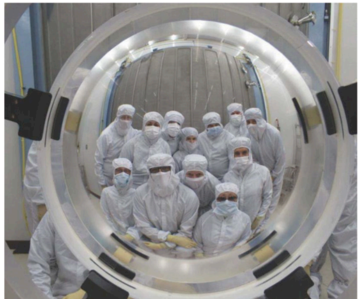
Figure 2. One of the six lenses of the new DESI corrector, which will give the Mayall telescope an 8-square-degree field of view, together with the crew who applied the anti-reflective coating. (Credit: Viavi Solutions)
