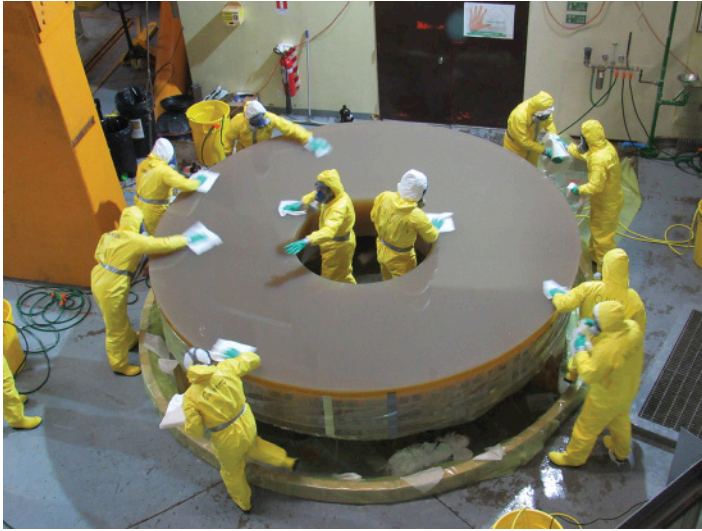
Figure 1. Cleaning the stripped surface of the primary mirror immediately before installation in the aluminizing chamber. (Credit: NOAO/AURA/NSF)
