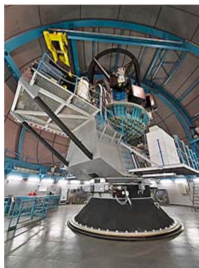
The Southern Astrophysical Research Telescope (SOAR), one of four 4m-class telescopes that are accessible through the NOAO proposal process.
