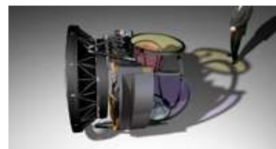
The LSST camera with its six filters (ugrizy). Five are in the filter wheel at any given time. (2011) (Image credit: Todd Mason, Mason Productions Inc. / LSST Corporation)
