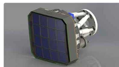
ZTF focal plane design - Sixteen 6.1k x 6.1k e2v CCDs, on a curved focal surface, covering 47 deg 2 .
