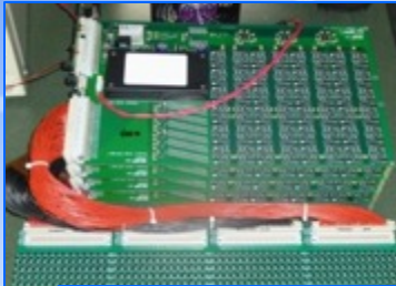
DM Electronics Prototype & CILAS DM 6x60 Breadboard test setup (warm) at NRC - Herzberg
