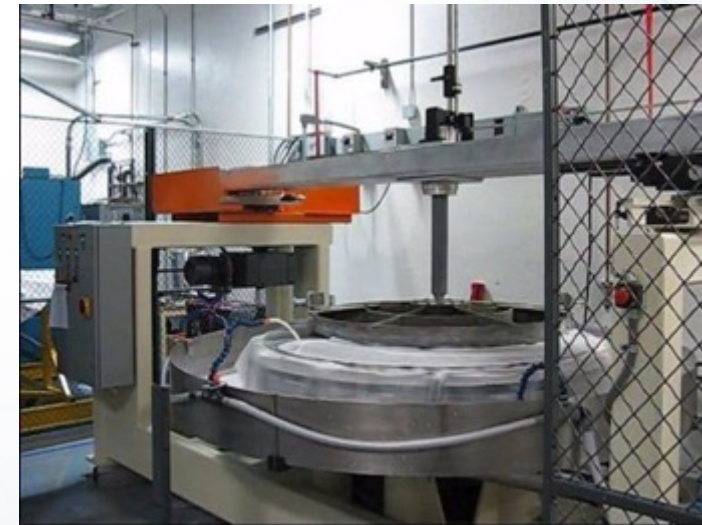
Polishing the stressed segment with a spherical tool
