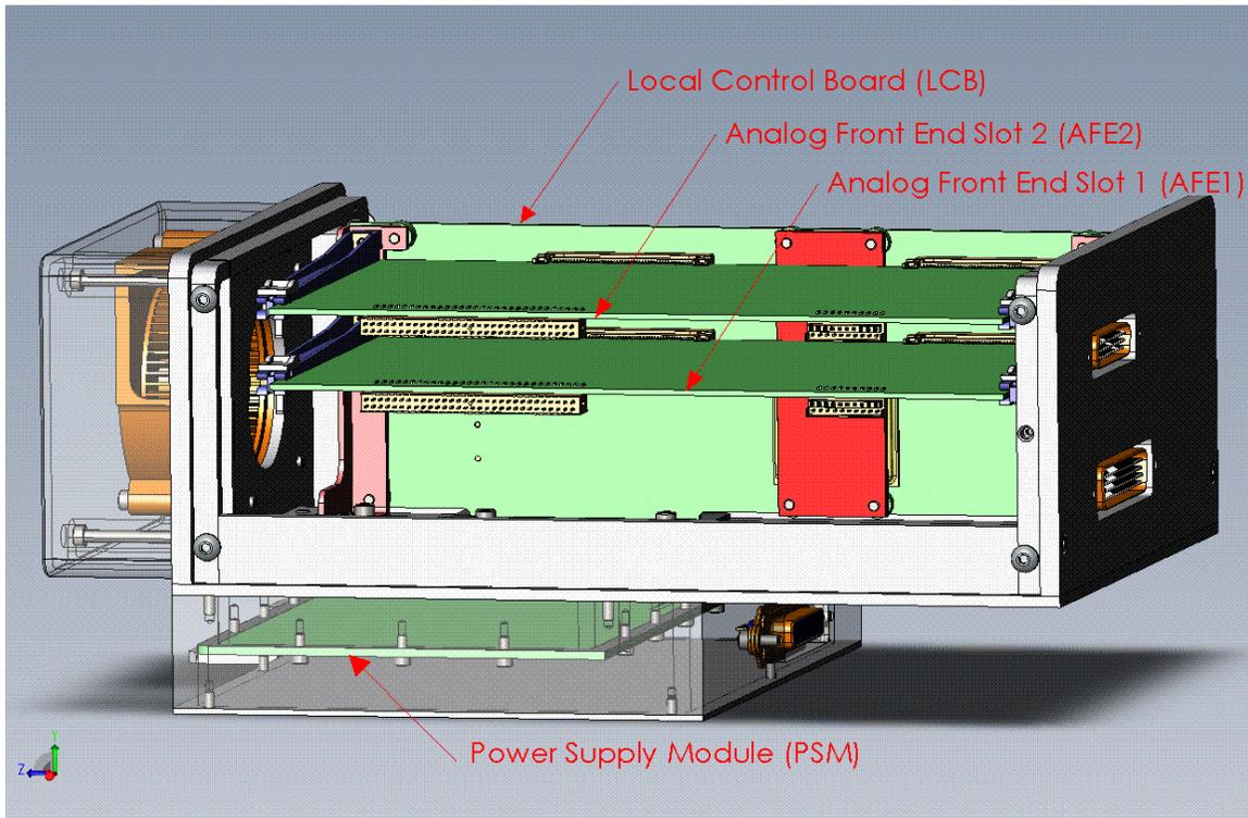
**Figure 2 - Torrent Transition Module**
