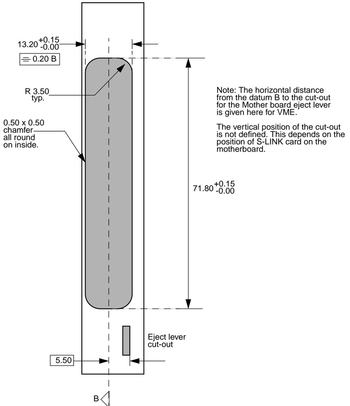
FIGURE 17. CMC bezel front panel (may be fitted to S-LINK cards if required)
