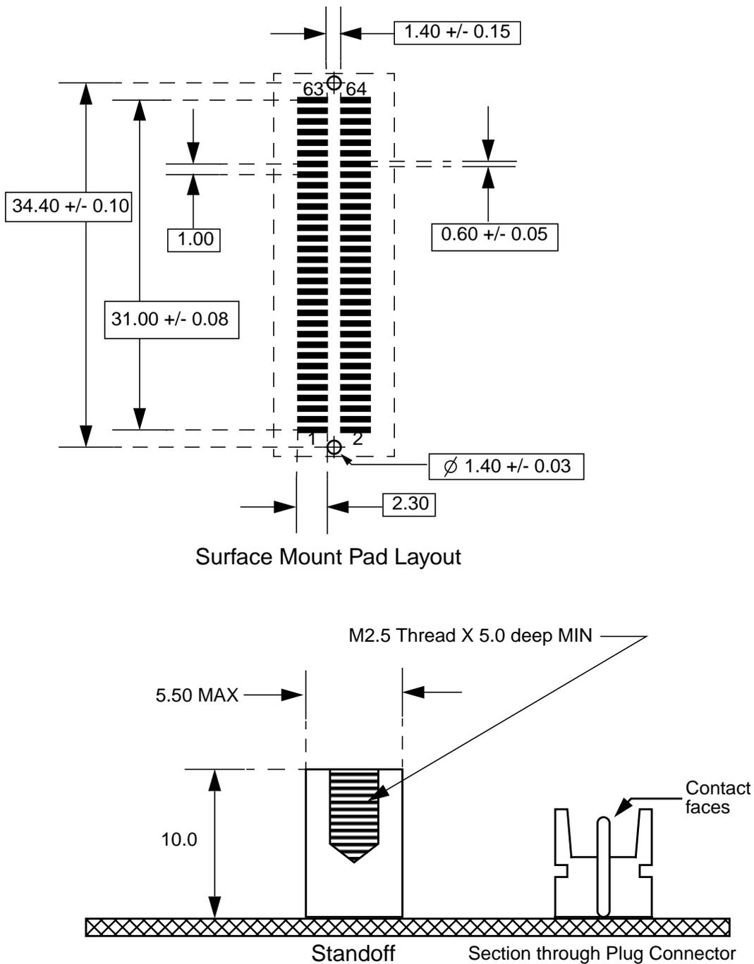
FIGURE 13. CMC "J" Receptacle Connector on motherboard
