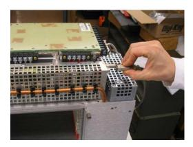
ii. Unplug orange left fan plenum power cable, (Cable C).
