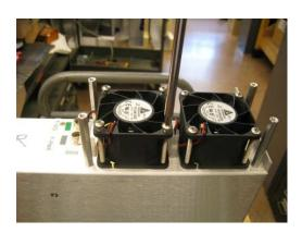
ix. Mount the fan shield to the Fan Plenum Module.
