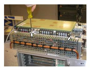
iii. Lift ICC Board Module straight up and remove.
