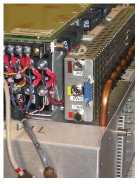
vii. Cables with Hirose connectors are unplugged by turning the connector counter-clockwise and pulling carefully until connector is unplugged.
