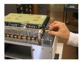
iii. Unplug grey right fan plenum power cable, (Cable C).
