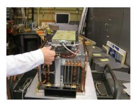
ii. Unplug violet Vicor Fan RPM cable, (Cable G).
