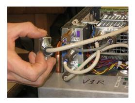
i. Unplug violet Vicor Fan RPM cable, (Cable G).
