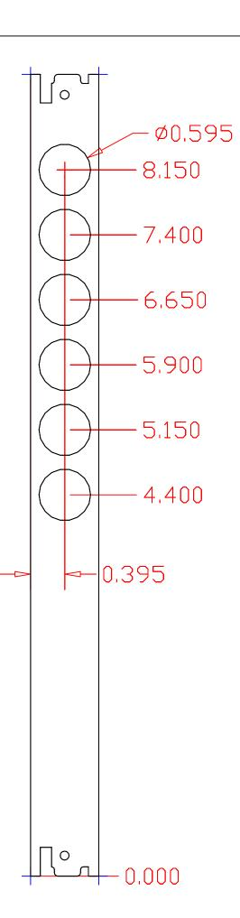
Caution: There are two orientations for front panels; note orientation of large slots is different (top-to-bottom) for Driver, Patch panel boards (20) and the mating transition boards (6).
