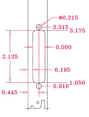
Caution: There are two orientations for front panels; note orientation of large slots is different (top-to-bottom) for Driver, Patch panel boards (20) and the mating transition boards (6).
