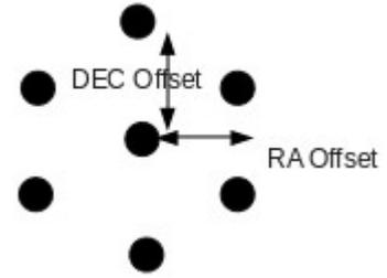
Note, equal RA and DEC offsets makes a slightly non-regular hexagon.
