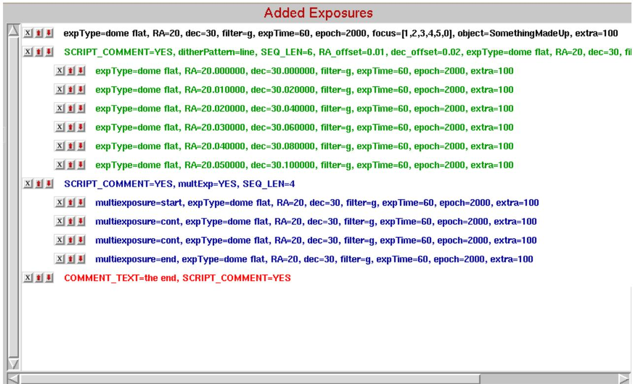
When an exposure is added, it is appended to the added exposures panel, which is pictured above. An exposure's line within the list displays that exposure as a string, as it would be passed to the OCS. Each line also includes three buttons. An 'X', and up and down arrows. The 'X' deletes the exposure from the queue, the up arrow moves the exposure up in the queue and the down arrow moves the exposure down in the queue.
