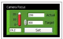
The *Actual* indicator box displays the current position of each lens system. To change the focus, the user may enter the desired position in the *Target* control box and click *Set*. If the desired position is outside the permitted range, the entered value will be coerced to the nearest acceptable value.
