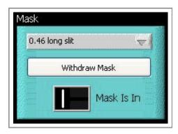
button will withdraw the slit from the beam path, revealing a 3' x 5' imaging field. With the slit withdrawn, the button will instead say 'Replace Mask.' Clicking this button will return the slit to the beam path. If no mask is desired, select the <*NO MASK*> option from the drop-down menu.
