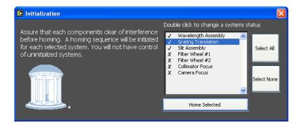
Once selections have been made, press the *Home Selected* button to initialize the motors. Immediately following this action, the indicator lights on the main GUI will turn from dark green (un-initialized state) to yellow (moving state). As each motor reaches its home position, the color of its indicator light will turn to light green (ready state).
