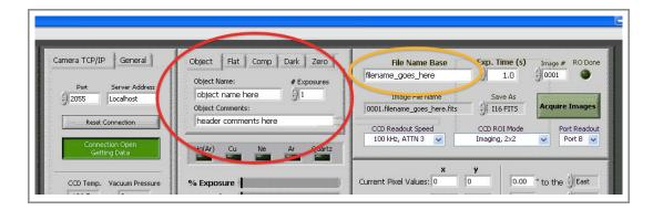
In the text box labelled *File Name Base*, enter the filename you would like for the image. Note that the software will add a number to the front of what is typed here and the ".fits" extension to the end.
