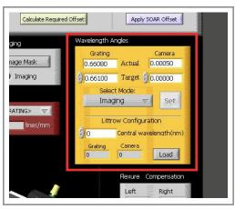
These angles will determine the range of wavelengths that falls on the CCD chip. There are three ways to do this:
