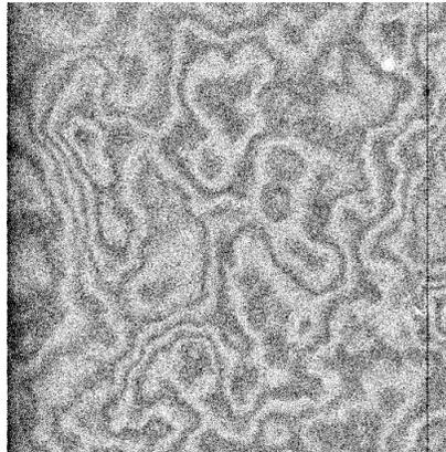
Figure 2.5: Example of the Mosaic-1 **fringe** pattern in a 512 x 512 pixel region. *This image needs to be updated for DECam data.*
