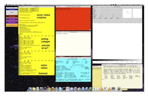
Figure 2: MacMini screen after completion of WildFire startup. The Engineering Daemon window is the red one at top. At the end of the initialization, a second beige Phoenix Daemon window will open up.
