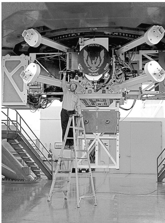
Figure 1. Phoenix mounted on the instrument support structure of Gemini South. K.H.H. is standing on the ladder under the instrument. Below his shoulder level is a standard Gemini instrument mounting frame for another instrument in the uplooking port. To his left, occupying a side looking port, is GCAL, the Gemini calibration unit. The end of the Phoenix dewar is prominent (behind the logo) with one cold head visible below the dewar. The four 'legs' are the balance weights required to match the weight and moment to the Gemini instrument specifications.
