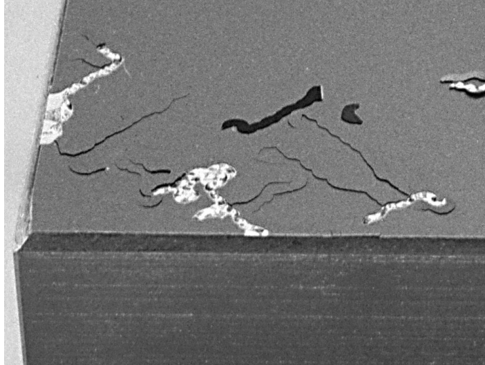
Figure 2. A close up of the corner of the silicon grating blank showing the debonding of the epoxy replica and the silicon substrate. The debonding fractures extended into the substrate. Debonding occurred mainly on the corners and to a much smaller degree along the edges of the grating. Debonding occurred in small areas on every thermal cycle. The grating surface shown here is approximately 5 cm wide by 3 cm deep.
