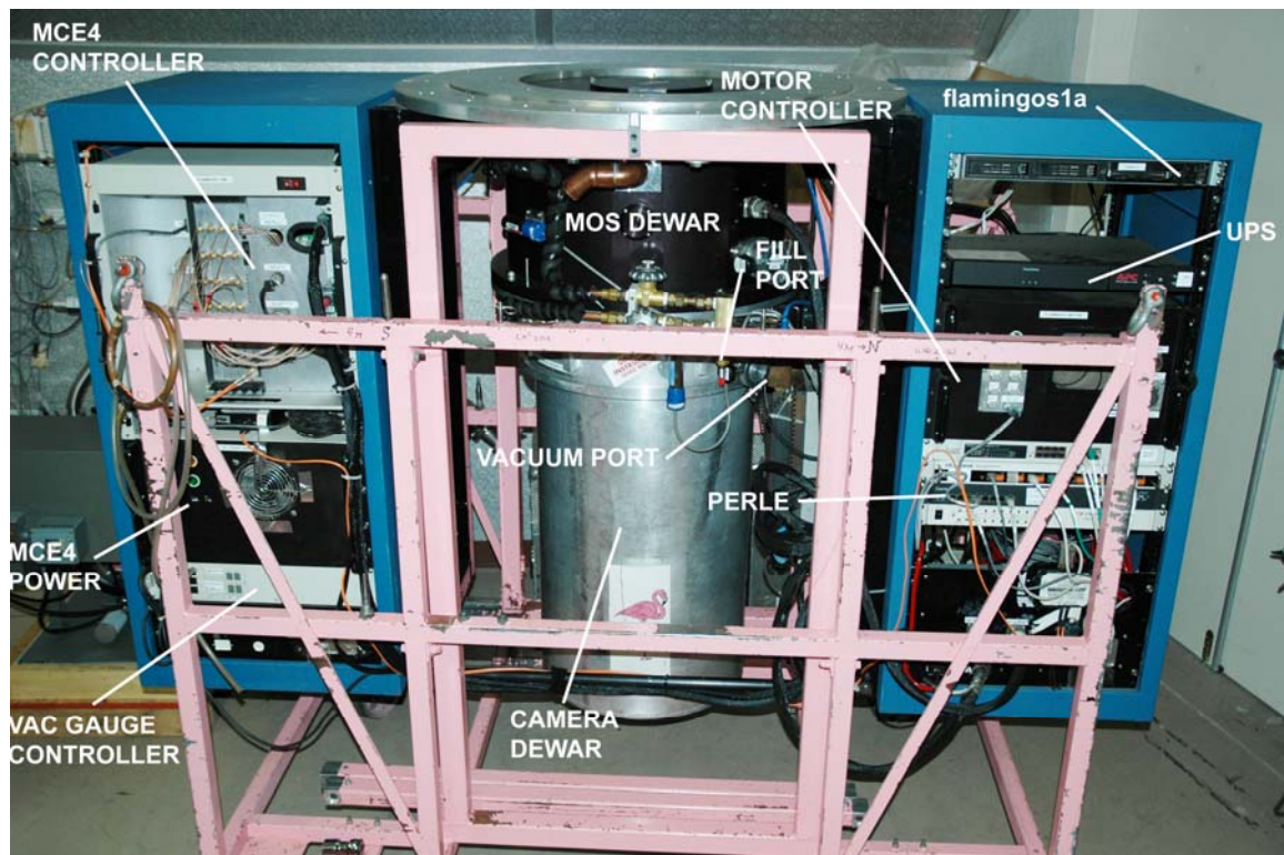
Figure 2: Front view of FLAMINGOS, showing the flamingos1a computer, UPS, Motor Controller, and MCE4 Detector Controller.
