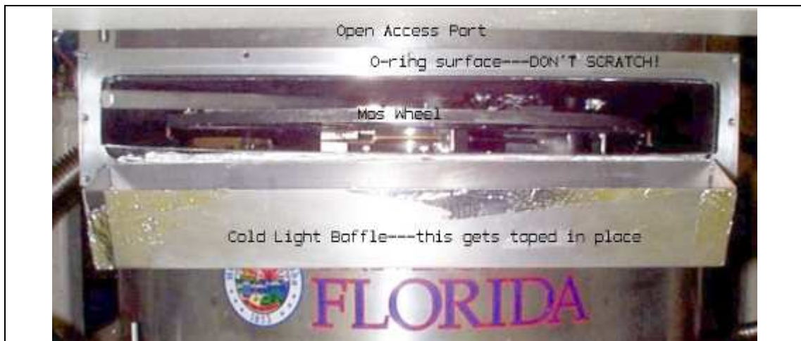
Figure 13. Open Mos Access Port. The Mos wheel and gear train are visible in the middle of the access port.
