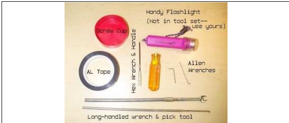
Figure 12. Useful Tools for Loading Mosplates. The hex wrench and handle have been replaced by a tool that does not come apart; it is used to take out the screws holding on the Mos access port cover. The Allen wrenches have been replaced by hex wrenches, one for each of the two sizes of screws for insert mosplates and frames; the wrenches are kept in the sack of screws. The Aluminum tape is used to hold the cold baffle on over the Mos wheel. The long-handled wrench and pick tool are used to remove and re-insert the Mos wheel. A flashlight is useful for seeing in to the Mos wheel mounting bolt.
