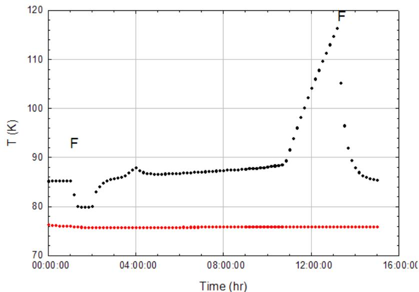
Figure 7: Temperature profile of the detector (red) and MOS work surface (black) over a 16 hour time period. The MOS dewar was filled (F) at about 0100, but the LN<sub>2</sub> ran out at about 1100. Note that the temperature rises approximately linearly at about 12 K/hr. The dewar was refilled at 1300 and required about 30 minutes to return to a normal operating temperature.
