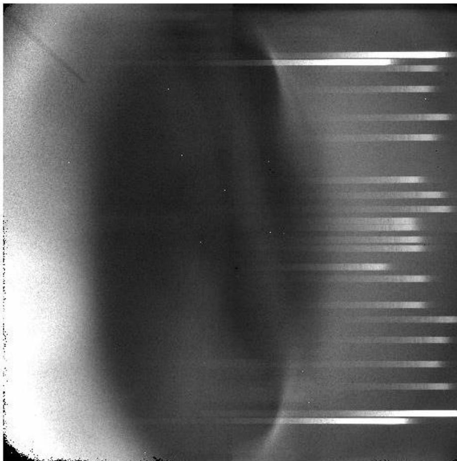
Figure 4: Raw image of a MOS spectrum in HK mode, showing the substantial dispersed thermal background superposed on the spectra of the MOS slitlets. The higher background spectra at the top and bottom are from the four square acquisition boxes on the MOS mask.
