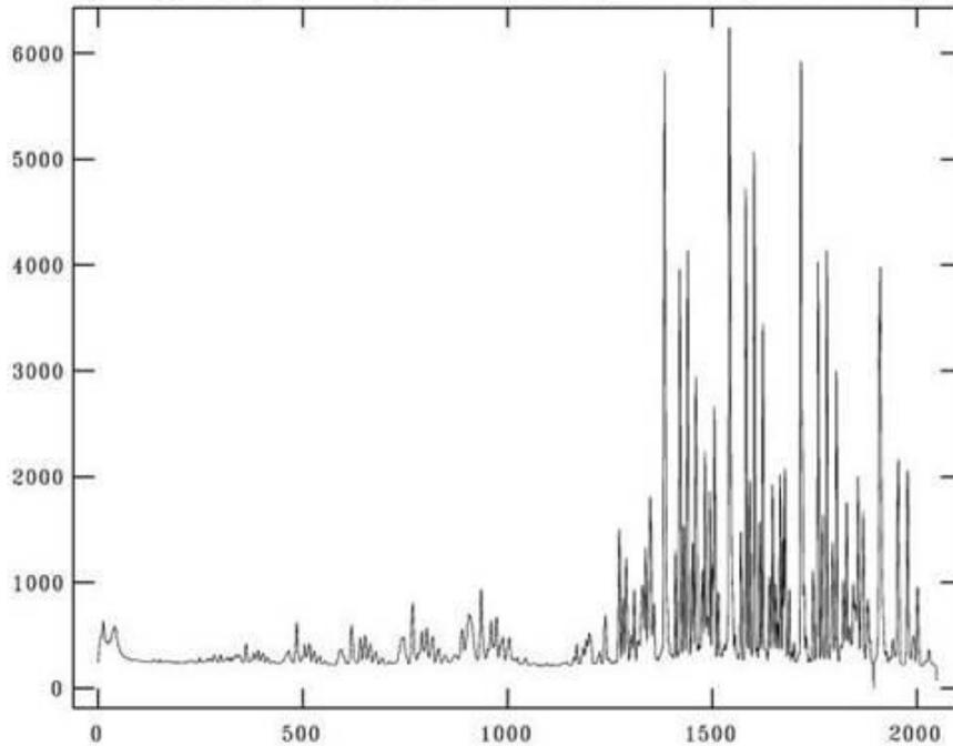
Figure 2: Plot of the JH sky spectrum from Fig. 1, showing the atmospheric OH emission lines. Signal is ADU (NREADS=1) in 600 s. Ordinate is in pixels.
