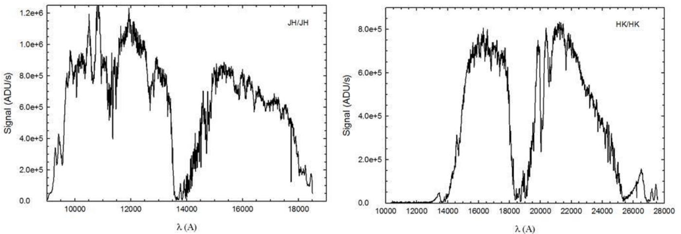
Figure 3: Raw FLAMINGOS signal levels in ADU/s for a 0.0 mag star through a wide slit for the JH region (left panel) and HK region (right panel). The signal in the HK spectrum redward of 2.5 microns is second order H band signal.
