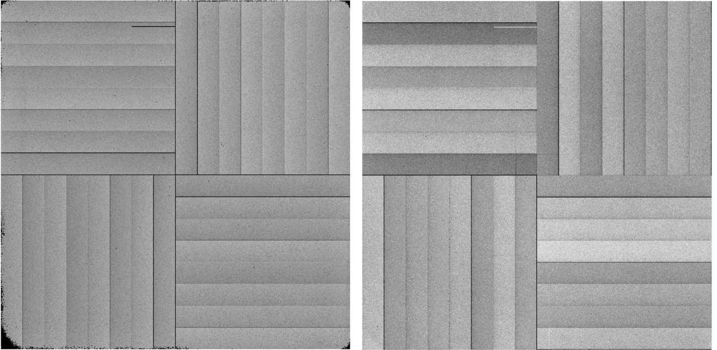
Figure 10: Representative FLAMINGOS images showing saturation due to excess radiation (left panel) and a "bad" read due to a premature readout of the array. Note that the dead pixels in the lower left corner show up clearly in the saturated image, but not in the bad read.
