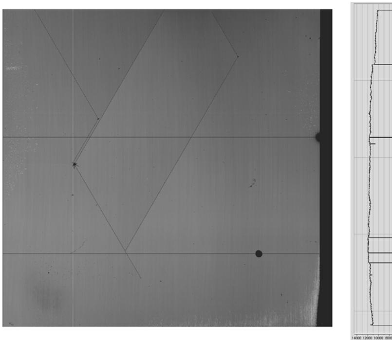
Fig. 1 PEDs, inoperable rows, diagonal cracks, and debonded corner on SN013.
