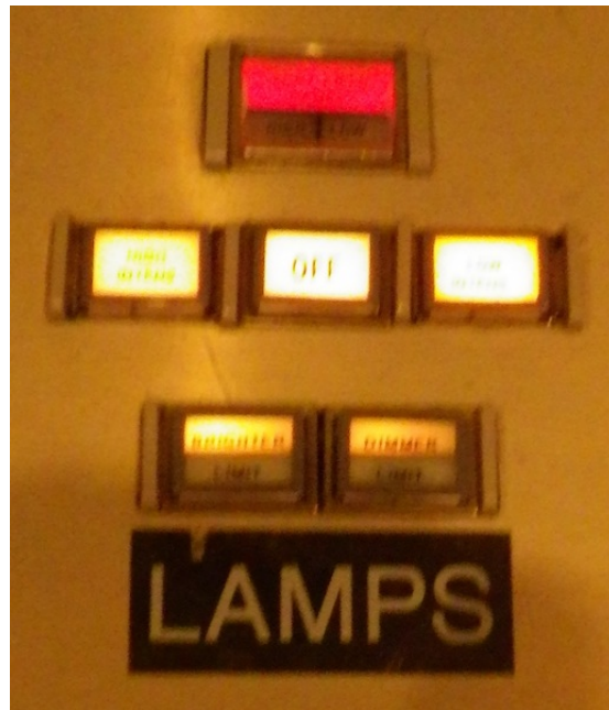
Fig. 35. Dome flat lamp pushbuttons with lamps off. The topmost display button does not show either high lamps or low lamps as "on".
