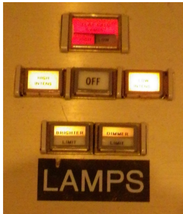
Fig. 36. Dome flat lamp pushbuttons with high lamps selected.
