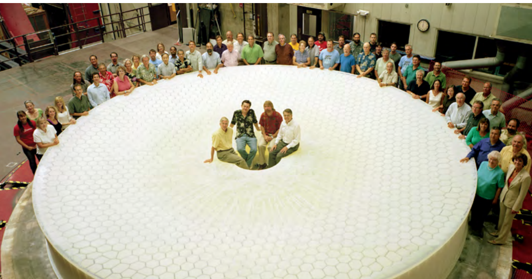
Team members celebrate the successful casting of the telescope's 27.5-foot-diameter mirror blank in August 2008. Credit: Howard Lester/NOIRLab/Vera C. Rubin Observatory/NSF/AURA
