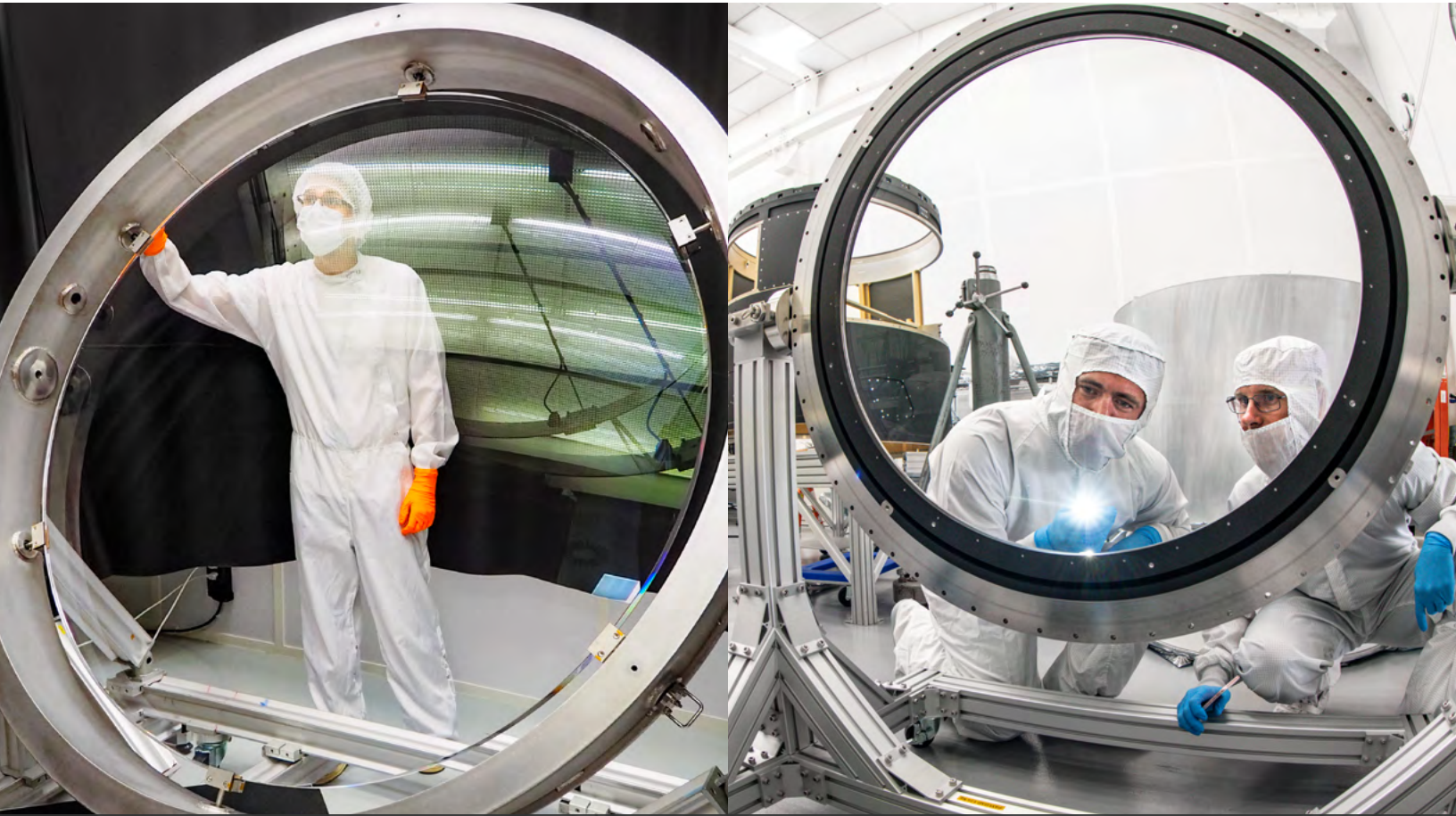
To the left, the photo shows the largest lens of the Vera C. Rubin Observatory camera. Credit: SAFRAN. To the right, the smallest of the three lenses. Credit: Jacqueline Orrell/SLAC National Accelerator Laboratory
