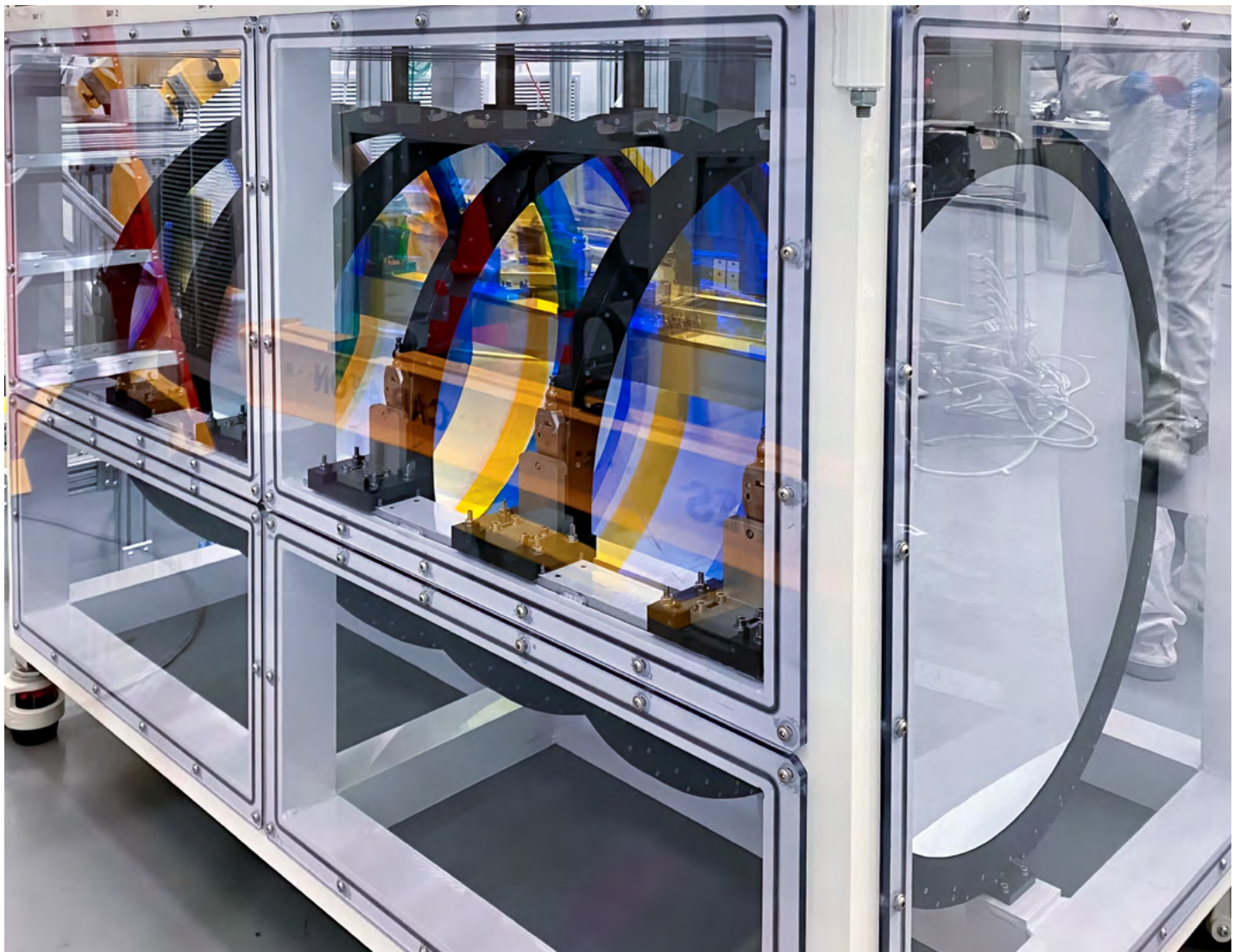
The six LSST Camera filters in their storage container at SLAC National Accelerator Laboratory, prior to shipping to Chile in May 2024. Credit: SLAC National Accelerator Laboratory
