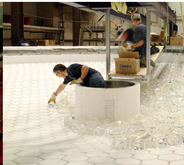
Chunks of glass are loaded during fabrication of Rubin Observatory's 8.4-meter combined primary/tertiary mirror. Credit: Ray Bertram/Rubin Observatory/NSF/AURA
