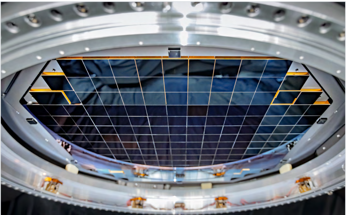
The complete focal plane of the LSST Camera is more than 60 cm (2 feet) wide and contains 189 individual sensors that will produce 3200-megapixel images. Credit: SLAC National Accelerator Laboratory
