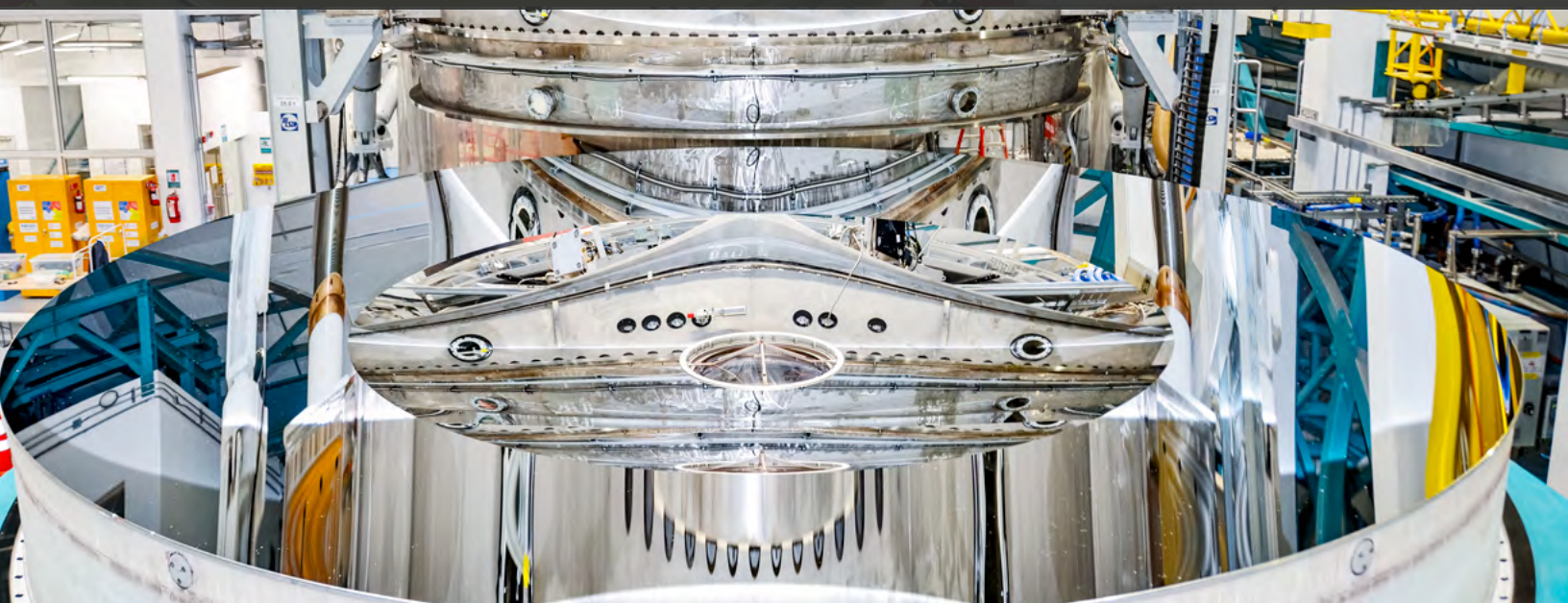
Rubin Observatory's 8.4-meter combined primary/tertiary mirror with its protected silver coating, applied in April 2024. Credit: Rubin Observatory/NSF/AURA
